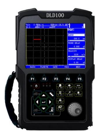
Rugged DLD100 durability, 10 hours of battery use, easy keys operation, outstanding ultrasonic performance, and now "square wave pulser" and "color leg" combine to form a powerful portable ultrasonic inspection tool with powerful Lithium Ion battery pack.
